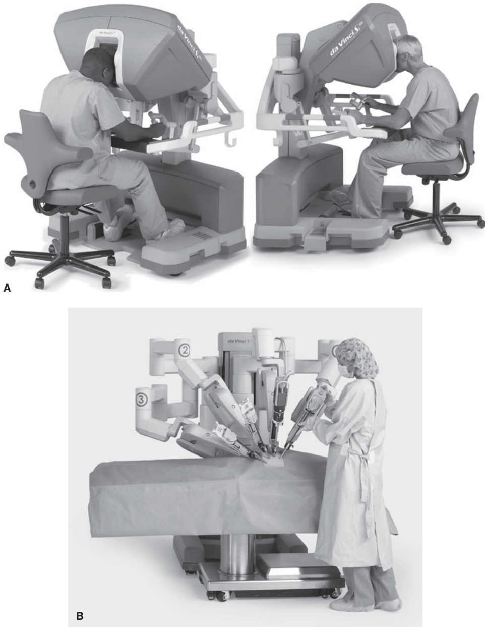
▲ Figure 10-1. The da Vinci Si robotic surgical system made by Intuitive Surgical Inc. It consists of the (A) surgeon console (here with the dual console HD Si) and (B) patient-side surgical cart, in this model with four arms (Images courtesy of Intuitive Surgical Inc.).
